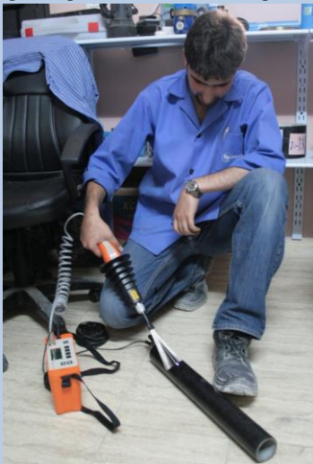
Checking for flaws on pipes in Hebron
